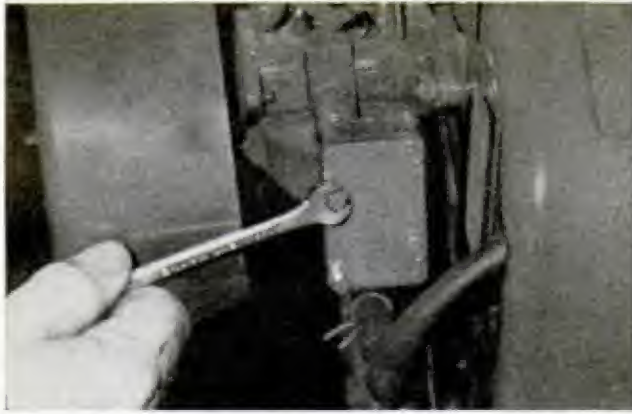
EXTERNAL FUEL PUMP "failure" may not be that. First tighten the bolts which may be admitting air
